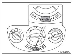
Press this button when driving in dusty conditions or to avoid traffic or outside fumes, and when quick cooling or heating of the passenger area is required. The indicator light will illuminate and interior air will be recirculated.
